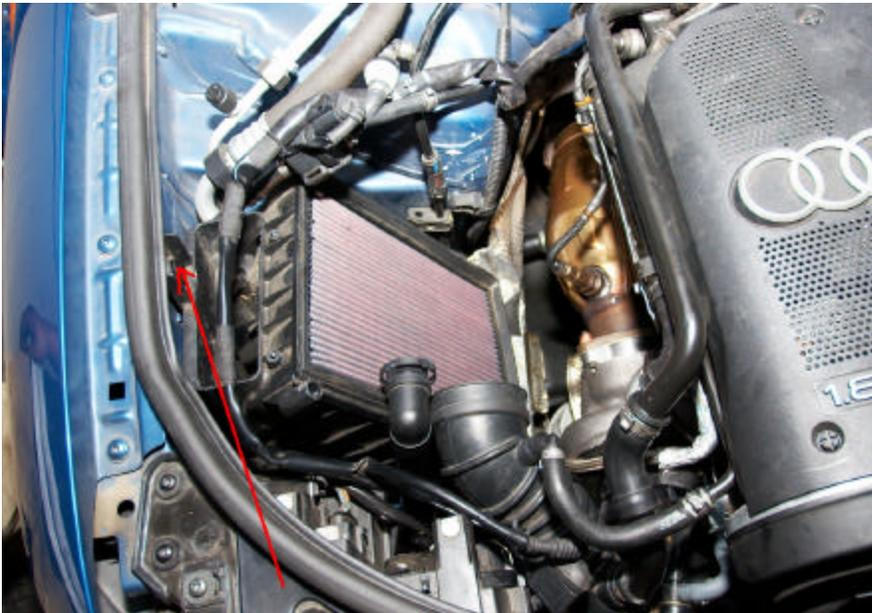
26. Reinstall the bottom half of air box along with the black plastic retaining pin.
