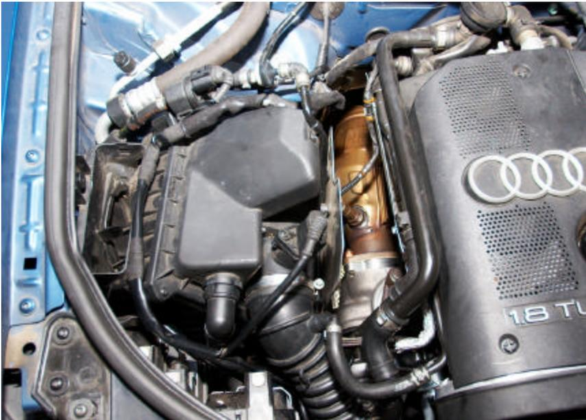
27. Reinstall the top half of air box in reverse order and tighten down two screws and all clamps.
