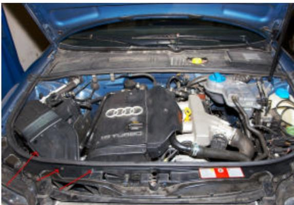
1. Remove two screws holding air box inlet duct in place.
