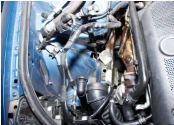
10. Remove bottom of air box from vehicle.
