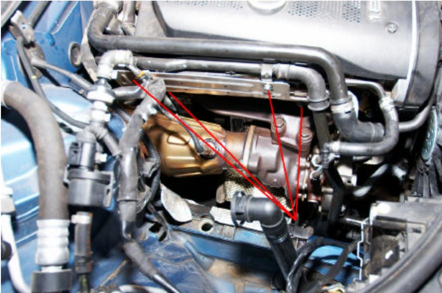
11. Remove the 4 (10mm) bolts holding the flat heat shield to the head.
