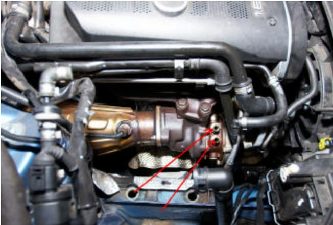
13. Unscrew the oil feed line and coolant feed line from top of turbo.
