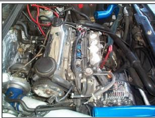
Attach upper inlet pipe (figure E) between turbo compressor outlet and lower inlet pipe. 13. Note: Cap off nipple with 3/4" vacuum cap if installing on OBD II engine. Nipple is only for use on OBD I engines with idle stabilizer.
