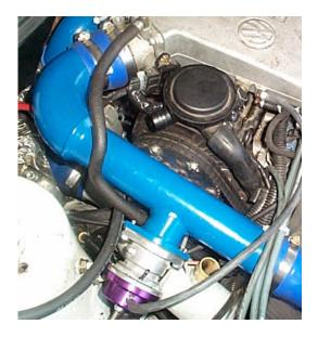
Connect Greddy or HKS Type S blow off valve to pretapped flange use (2) 1/4" corse 15. thread bolts, ensuring gasket is in place. Tee boost line into boost signal on BOV.
