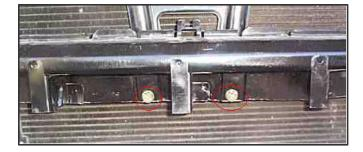
10. Place intercooler assembly bracket by aligning top brackets to open holes from bolts:
