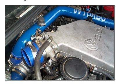
14. Install upper outlet pipe (figure A) between throttle body and lower outlet pipe:
