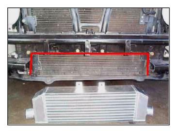
9. Using 13mm socket, unbolt the two support bolts near the center:
