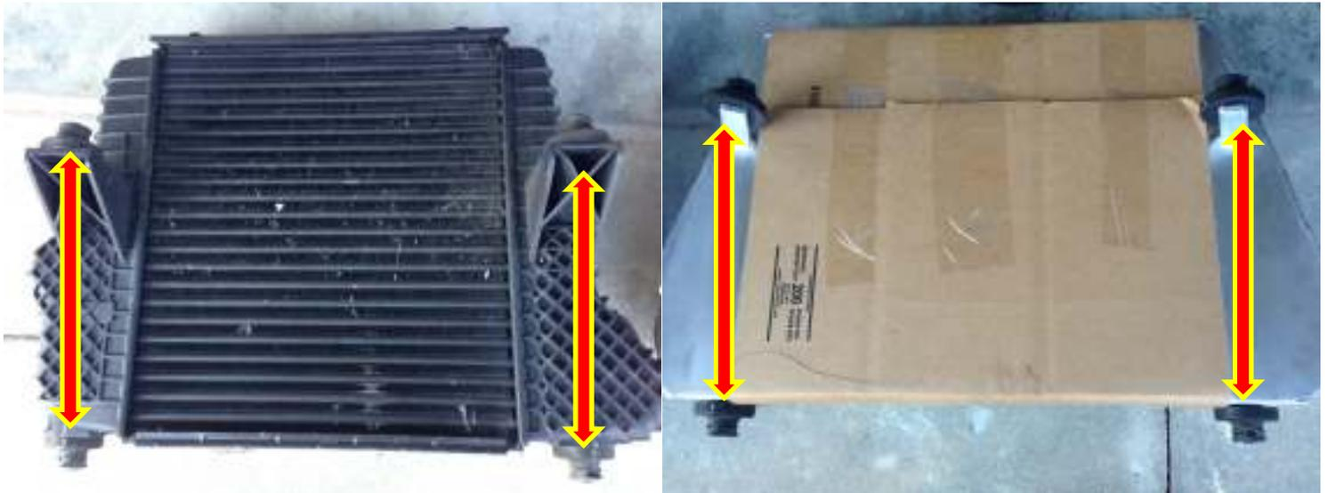
10. Reinstall Lower CAC bracket using 13mm socket and Lower Rear Valance if removed with 15mm deep socket and tighten it up. (The new CAC can be installed from above)
