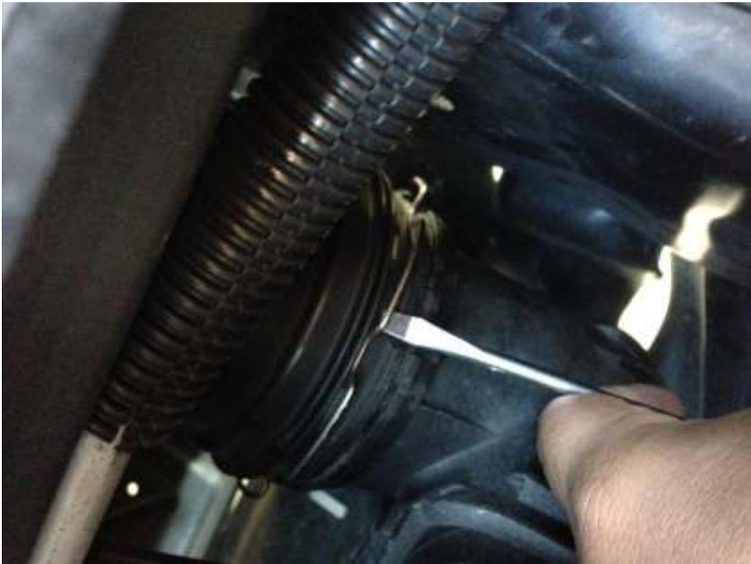
**NOTE: It may be easier to remove drivers side access panel to help remove clip from underneath connection. To do this Turn 4ct white clips ¼ turn Counter-clockwise till they release.**
