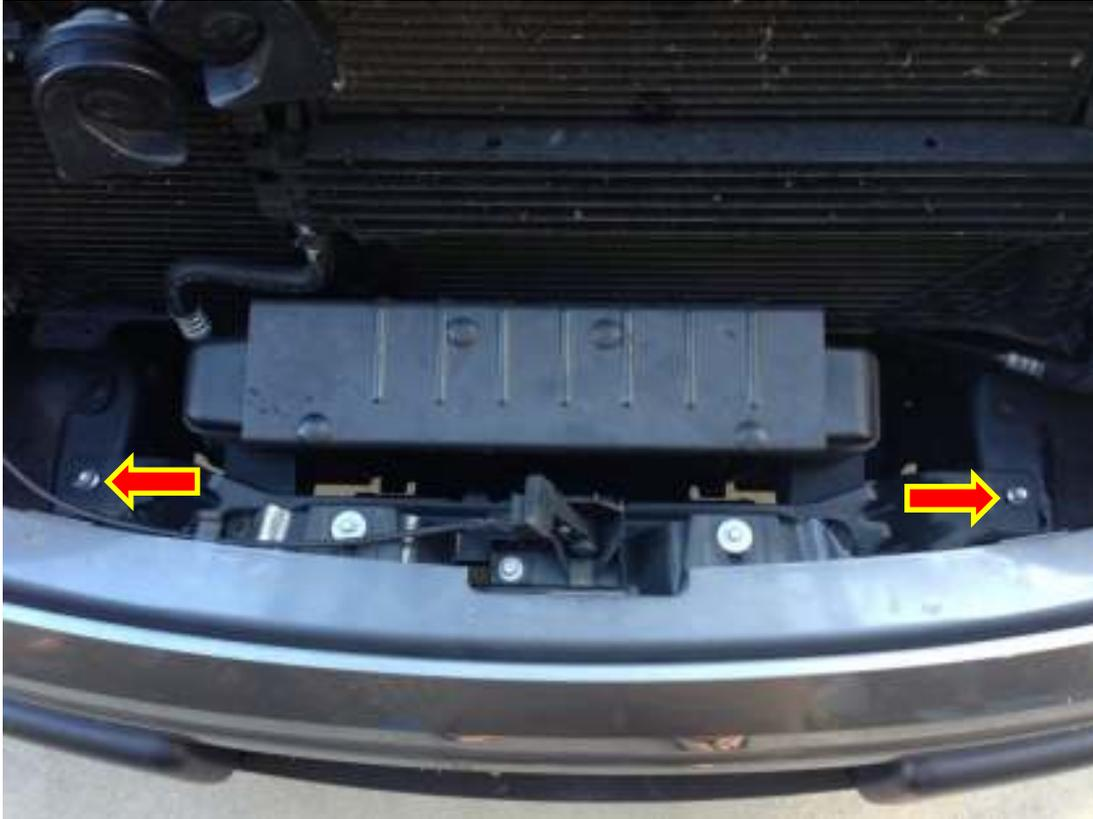
2. Remove Upper CAC Bracket and put aside. Good practice is to reinstall the bolts into the holes so they do not walk off.
