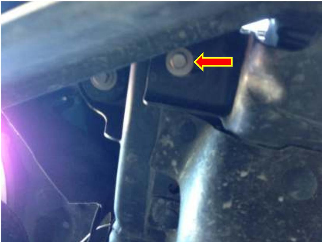
**NOTE: I found it easier to remove the rear lower valance to help get the CAC out but it is not necessary. If you opt for this you will need a 15mm deep socket to remove the nuts from the studs holding it on.**
